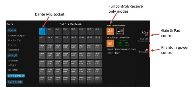
With a Dante DMI 64@96 card installed in a console, access to 64 channels of IO to/from the Dante network is provided.
